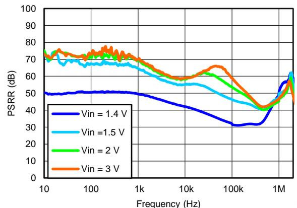
**Figure 43. POWER-SUPPLY REJECTION vs INPUT VOLTAGE**
