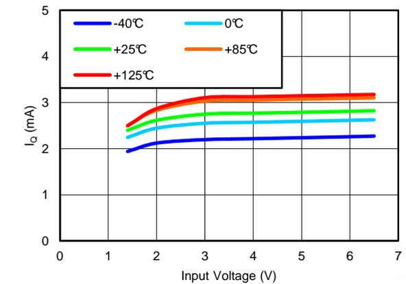
**Figure 19. GROUND CURRENT vs INPUT VOLTAGE**
