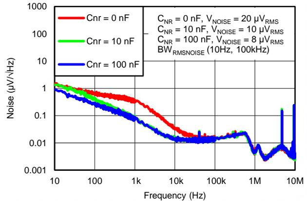
**Figure 45. SPECTRAL NOISE DENSITY vs  $C_{NR/SS}$**
