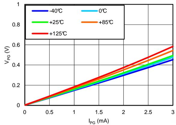
**Figure 37. PG LOW VOLTAGE vs PG CURRENT**
