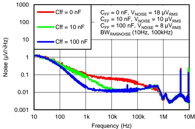
**Figure 46. SPECTRAL NOISE DENSITY vs  $C_{SS/NR}$**
