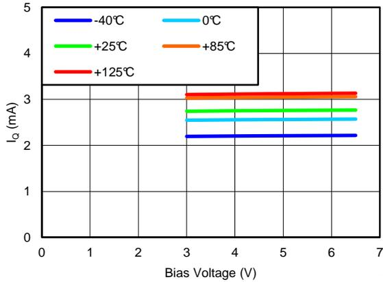
**Figure 20. GROUND CURRENT vs BIAS VOLTAGE**
