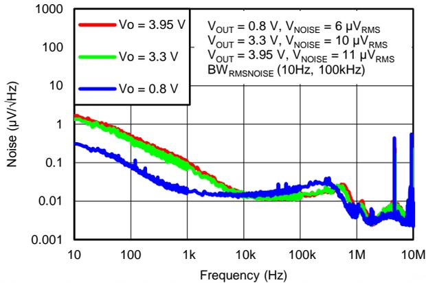
**Figure 44. SPECTRAL NOISE DENSITY vs OUTPUT VOLTAGE**
