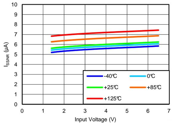
**Figure 25. SOFT-START CURRENT vs INPUT VOLTAGE**
