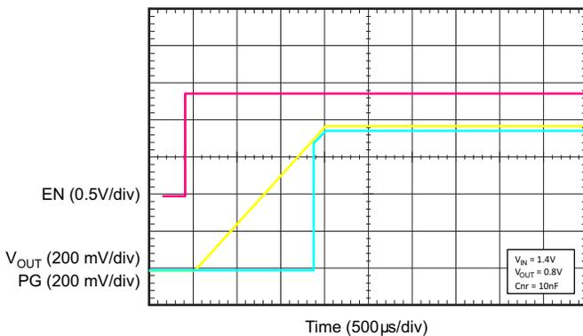
**Figure 49. START-UP ( $C_{NR} = 10\text{ nF}$ )**
