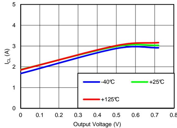
**Figure 29. CURRENT LIMIT vs OUTPUT VOLTAGE**
