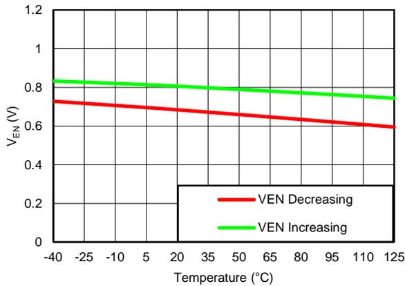
**Figure 34. ENABLE THRESHOLD vs TEMPERATURE**
