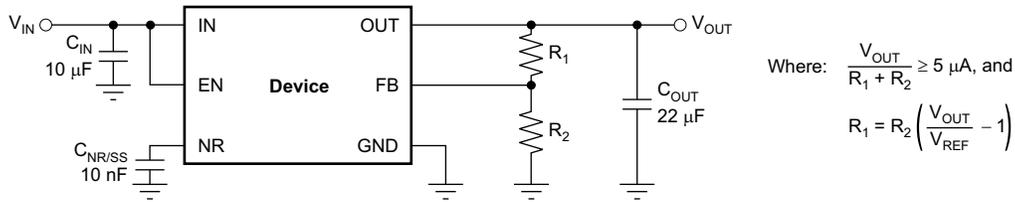
**Figure 52. Adjustable Operation for Maximum AC Performance**
