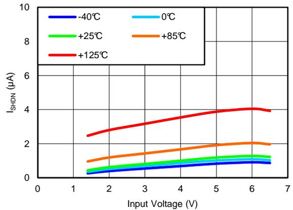
**Figure 23. SHUTDOWN CURRENT vs INPUT VOLTAGE**
