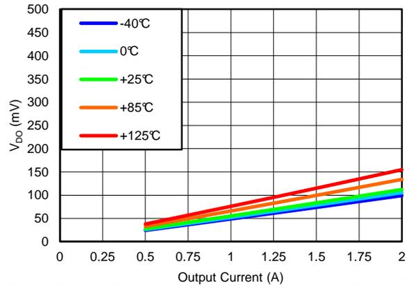
**Figure 13. DROPOUT VOLTAGE vs OUTPUT CURRENT**
