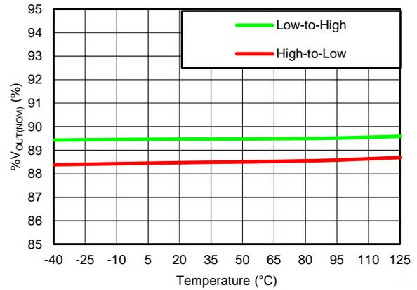
**Figure 39. PG THRESHOLD vs TEMPERATURE**
