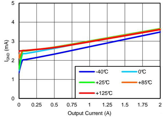
**Figure 21. GROUND CURRENT vs OUTPUT CURRENT**
