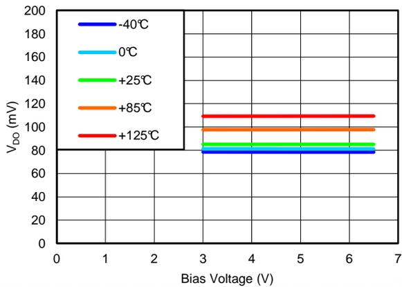
**Figure 18. DROPOUT VOLTAGE vs BIAS VOLTAGE**
