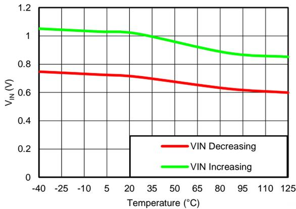
**Figure 30. INPUT UVLO THRESHOLD vs TEMPERATURE**
