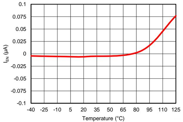
**Figure 35. ENABLE CURRENT vs TEMPERATURE**
