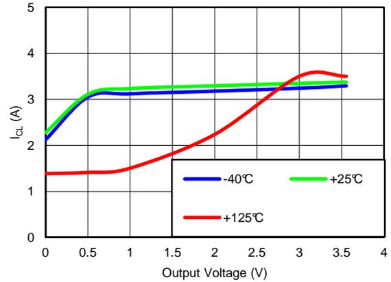
**Figure 27. CURRENT LIMIT vs OUTPUT VOLTAGE**
