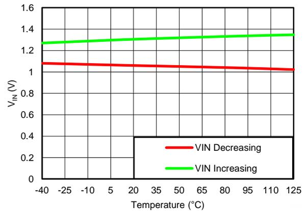
**Figure 31. INPUT UVLO THRESHOLD vs TEMPERATURE**
