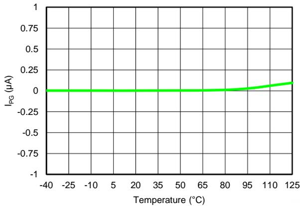
**Figure 40. PG CURRENT vs TEMPERATURE**
