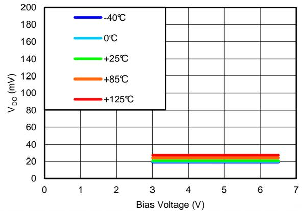
**Figure 17. DROPOUT VOLTAGE vs BIAS VOLTAGE**
