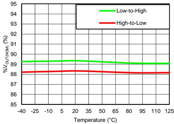
**Figure 38. PG THRESHOLD vs TEMPERATURE**
