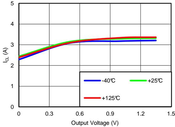
**Figure 26. CURRENT LIMIT vs OUTPUT VOLTAGE**
