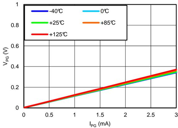
**Figure 36. PG LOW VOLTAGE vs PG CURRENT**
