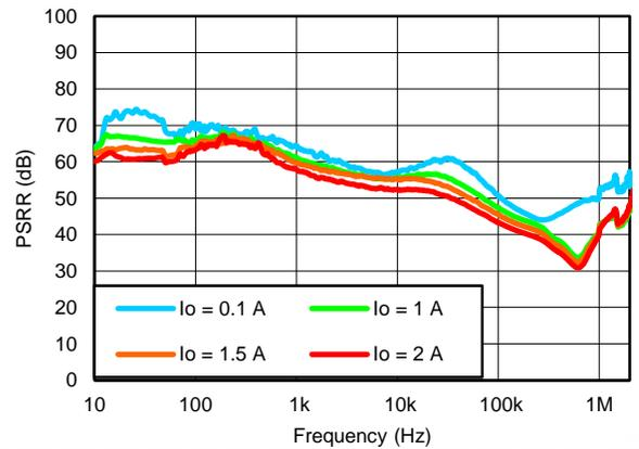
**Figure 41. POWER-SUPPLY REJECTION vs CURRENT**
