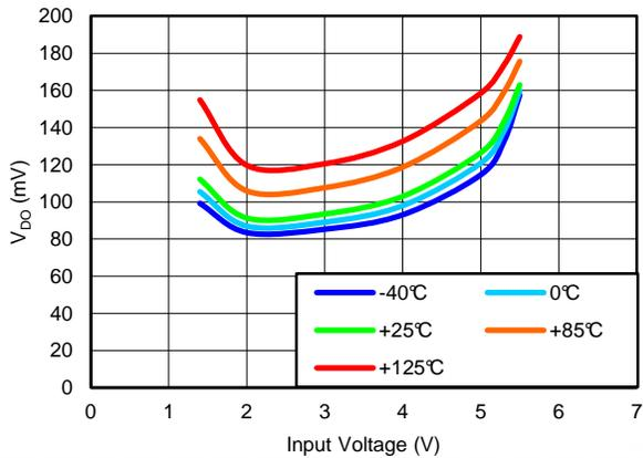
**Figure 16. DROPOUT VOLTAGE vs INPUT VOLTAGE**
