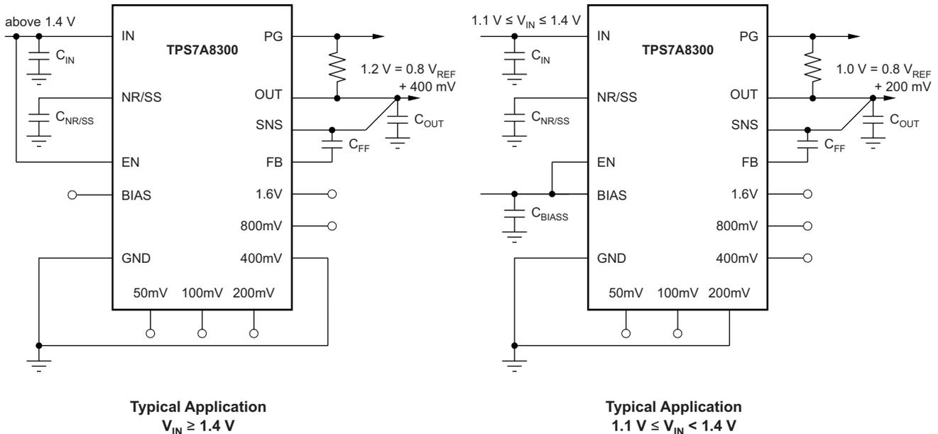
Figure 51. Maximize PSRR Performance and Minimize RMS Noise
