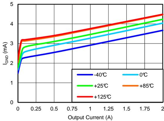
**Figure 22. GROUND CURRENT vs OUTPUT CURRENT**
