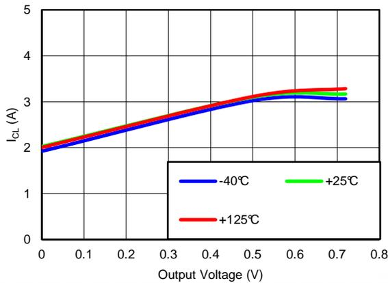
**Figure 28. CURRENT LIMIT vs OUTPUT VOLTAGE**
