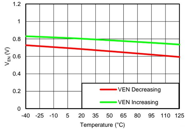
**Figure 33. ENABLE THRESHOLD vs TEMPERATURE**
