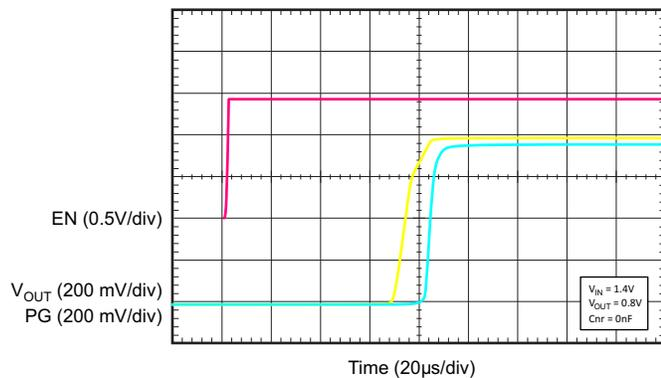
**Figure 48. START-UP ( $C_{NR} = 0\text{ nF}$ )**
