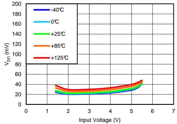
**Figure 15. DROPOUT VOLTAGE vs INPUT VOLTAGE**
