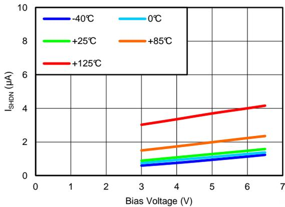
**Figure 24. SHUTDOWN CURRENT vs BIAS VOLTAGE**
