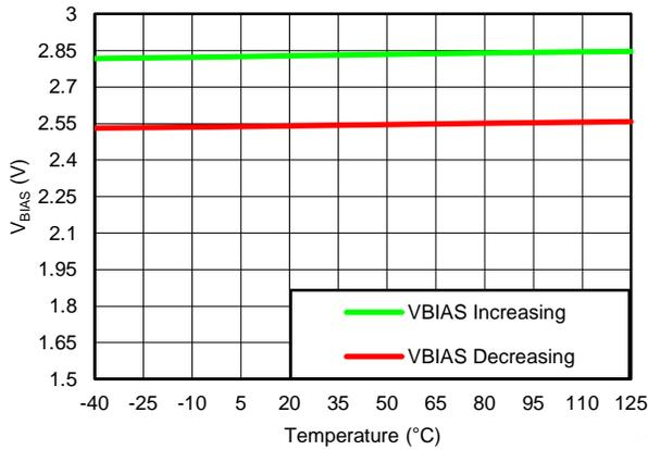
**Figure 32. BIAS UVLO THRESHOLD vs TEMPERATURE**
