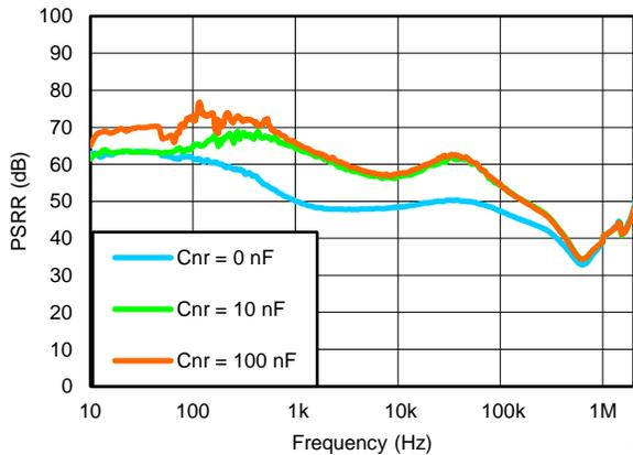
**Figure 42. POWER-SUPPLY REJECTION vs  $C_{NR/SS}$**
